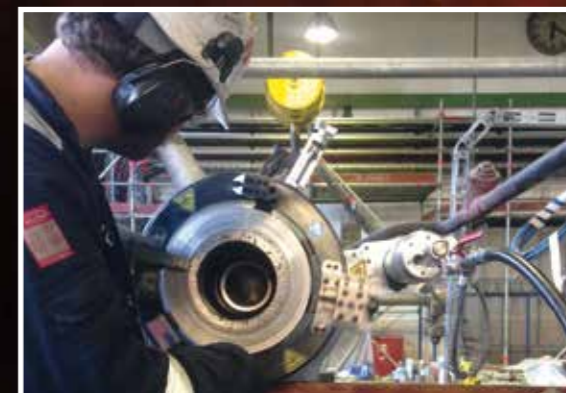
Bevelling 60 mm wall thickness.
